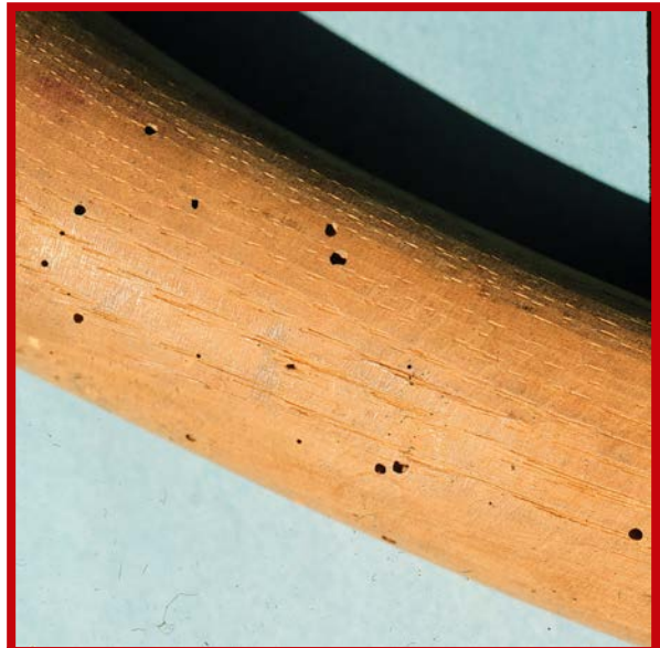
Emergence holes in wood.
